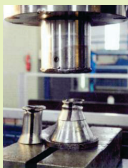
Flaring test > 20% of diameter
