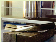
Flattening test 0° and 90°
