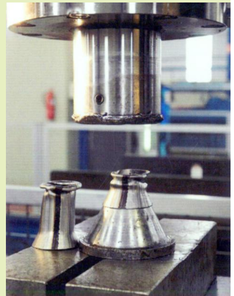
Flaring test > 20% of diameter
